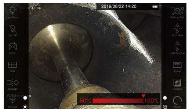
3 stage temperature warning & auto shut down function
